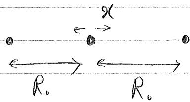
$$V_{(n)} = \frac{Z^2 e^2}{R_0 - n} + \frac{Z^2 e^2}{R_0 + n} \quad (|n| < R_0 - R_n)$$
